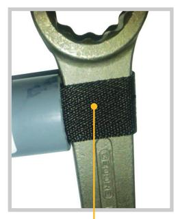
Inspect holding strap for excessive wear, damage caused by possible hammer strikes and tears. Slight fraying is acceptable.
