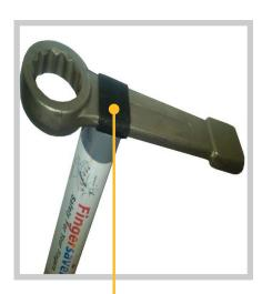
Attach the flogging (slogging) spanner to the Fingersaver using the holding strap.
