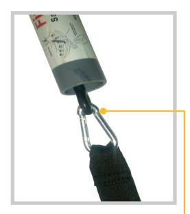
Inspect steel safety holding clip for excessive wear. This part is housed inside the outer shell and connects the tensioner and holding strap.
