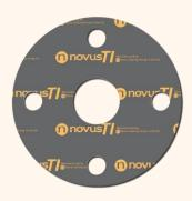
Novus TI is a graphite laminate product reinforced with an insertion of tanged O.10mm thick 316 stainless steel. No adhesive is required to bond the graphite layers to the tanged insert resulting in a sturdy gasket material with excellent mechanical strength.
