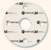
Novus 34 is a superior performance universal compressed sheet material based on a blend of aramid/inorganic fibres and special additives, with high quality Nitrile Rubber binder system.
